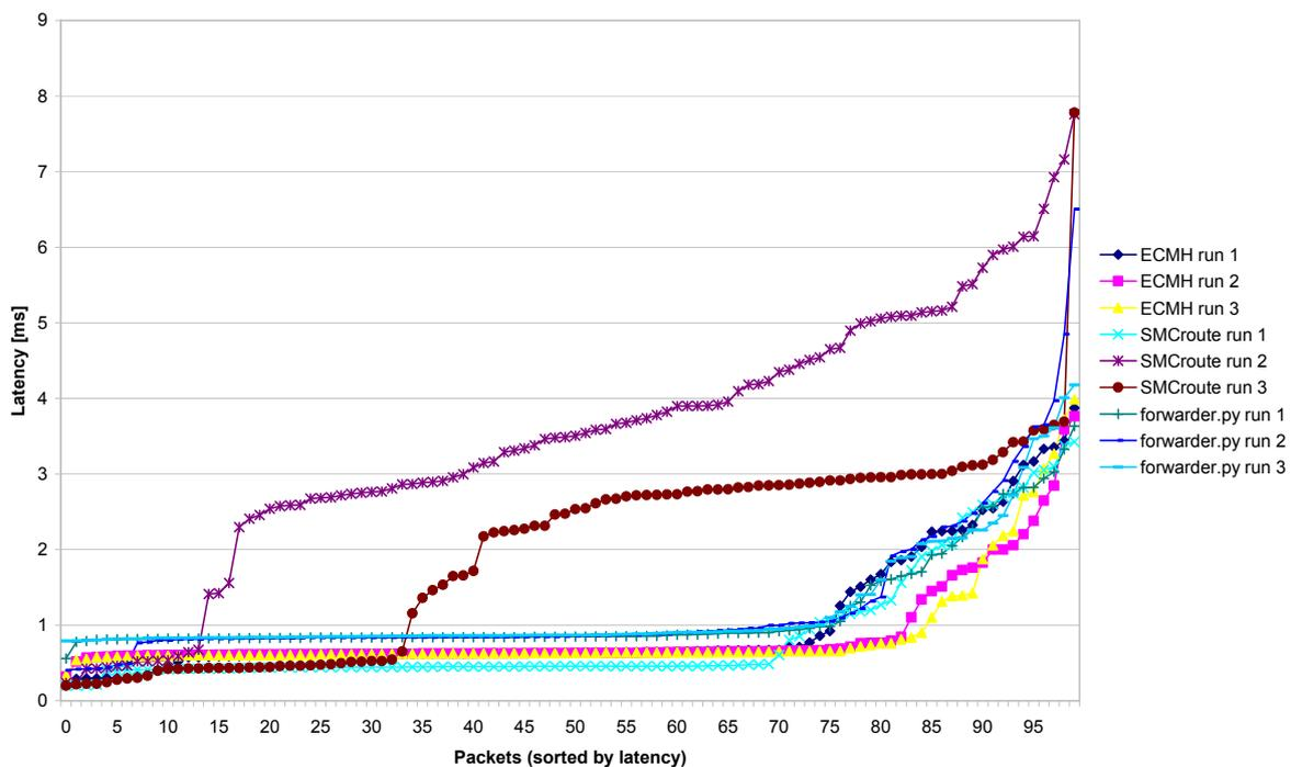
Figure 15: Internal latency in proxy implementations
