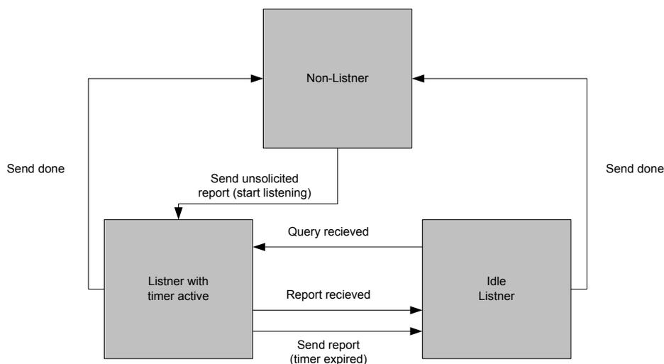
Figure 12: MLD state machine (adapted from [RFC2710])
