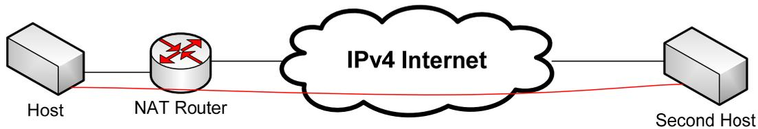
Figure 4: Semantic illustration of the AYIYA tunneling protocol (with the lower red line indicating the tunnel and the black lines indicating the actual network links)
