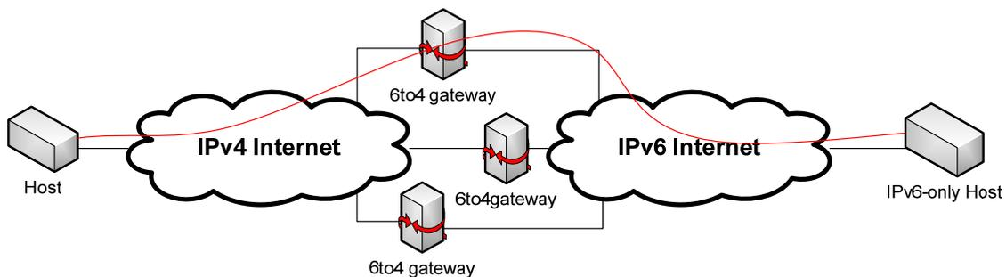
Figure 6: Semantic illustration of the 6to4 tunneling protocol (with the upper red line indicating the tunnel and the black lines indicating the actual network links)
