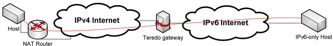
Figure 8: Semantic illustration of the Teredo tunneling protocol (with the lower red line indicating the tunnel and the black lines indicating the actual network links)
